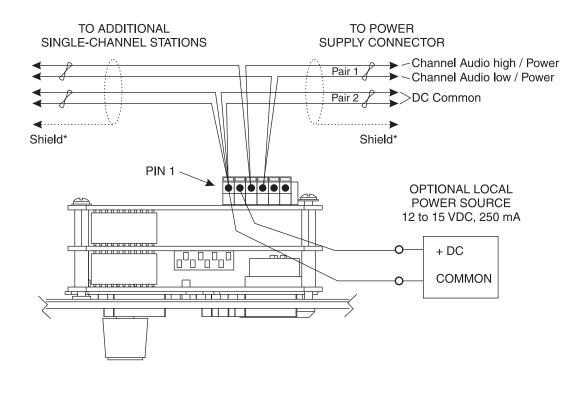
Cable Type: 22AWG Stranded, 2-Pair Twisted-wire, with Shield
